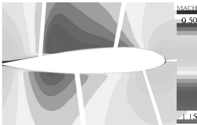
Fig. 18 BWB baseline configuration at M = 0.85 , C_L = 0.41 . Mach distribution at symmetry section z = 0.0 m.
