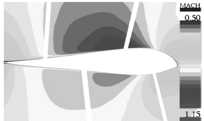
Fig. 19 BWB configuration. Multipoint optimization (case BWB\_3 ) at M = 0.85 , C_L = 0.41 . Mach distribution at symmetry section z = 0.0 m.
