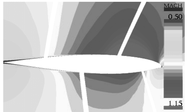
Fig. 21 BWB configuration. Multipoint optimization (case BWB\_3 ) at M = 0.85 , C_L = 0.41 . Mach distribution at section z = 13.0 m.
